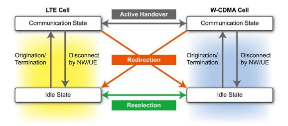
Figure 3. Case of UE Connection Cell in LTE and W-CDMA
