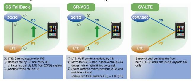
Figure 4. Technology Linked with 2G/3G System Circuit Switching
